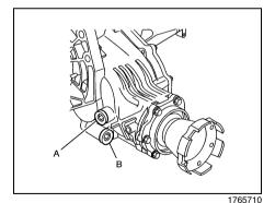
A. Fill Plug B. Drain Plug To get an accurate reading, the vehicle should be on a level surface.
